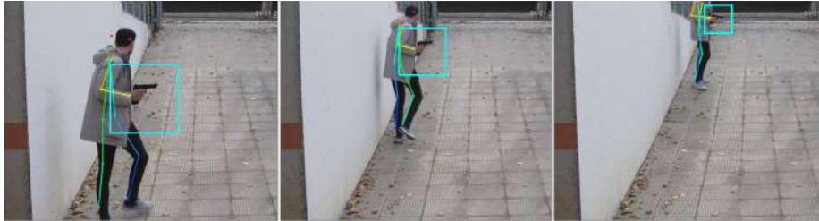
Figure 2: Illustration of how the Adaptive Pose Factor adapts the hand regions (i.e., the bounding box in blue color) at different distances from the camera. The further the smaller.
