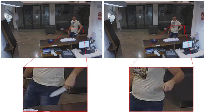
Fig. 10. Examples of blurry and noisy areas (indicated by red boxes) due in part to sudden movements in two frames extracted from a surveillance video. (For interpretation of the references to color in this figure legend, the reader is referred to the web version of this article.)
