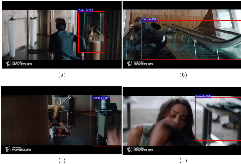
Fig. 1. Examples of false positives detected in the background, (a) a handbag in a showcase, (b) the mechanical stairs, (c) a screen and a laptop under a table and (d) an open case under a table.
