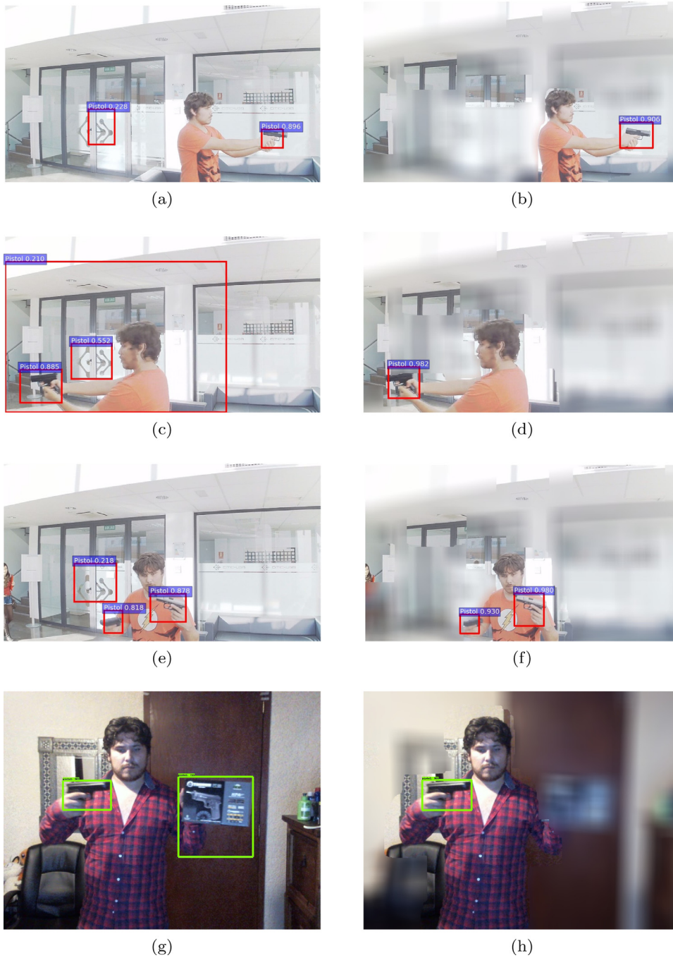
Fig. 5. Examples of the detection results with the proposed binocular image fusion, (b), (d), (f), (h) and without image fusion, (a), (c), (e), (g).
